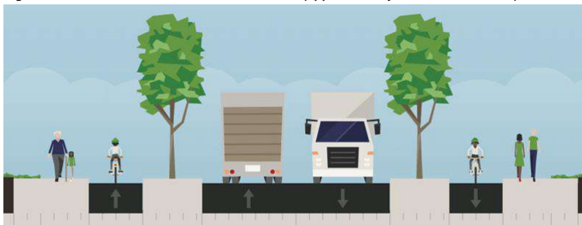
Figure 8-14: Indicative Two Lane Collector Road (approximately 21m Road Reserve)
